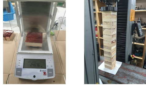
Fig. 2. Glue spread measurement and specimen press.
