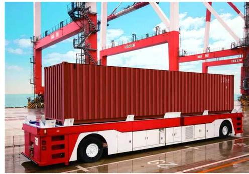
[Fig. 2] Port Container AGV
