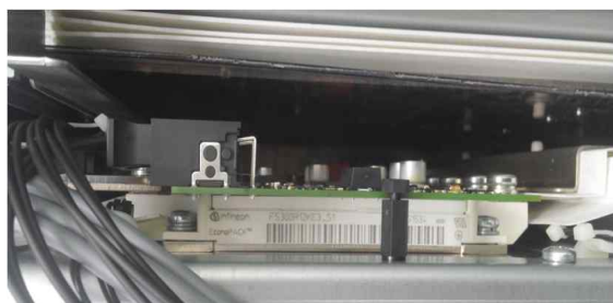
[Figure 12] IGBT of motor control
