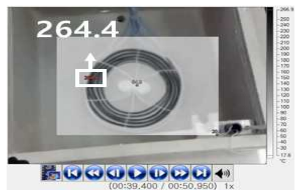
[Figure 10] Maximum temperature on thermo-graphic camera in experiment on improved plating equipment
