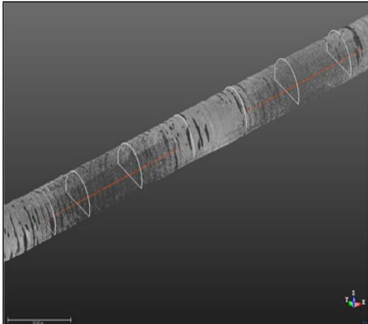
Fig. 8. Overlap of scanning data and designed data
