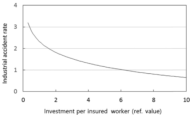
Fig. 1. IAR as a function of investment per insured worker as calculated by Eq. (2). Investment per insured worker y in Eq. (2) is a reference value and constant c and was arbitrarily set to best fit the simulation results to actual data in 2011. IAR, industrial accident rate.
