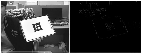
Fig. 8. Result of Canny Edge Algorithm
