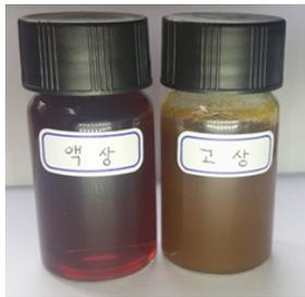
Fig. 4. Liquid and solid of lignin extract after separation.
