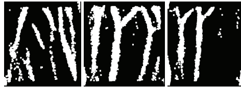
Fig. 9. Vein binary image after dilatation window (7×7).
