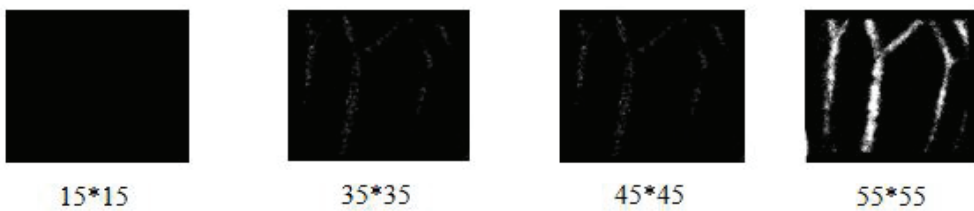
Fig. 6. Binarization by integral image for the extraction of dorsal hand veins.
