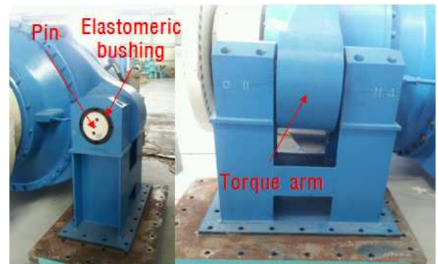
Fig. 2 Feature of torque arm of gearbox housing
