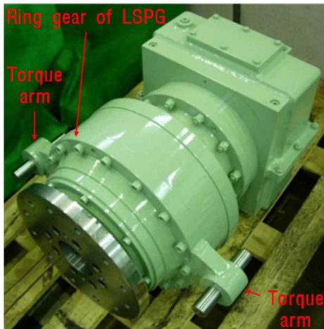
Fig. 4 Location of torque arm in the conventional type gearbox
