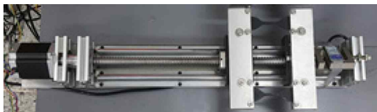
(b) Apparatus to stretch rubber specimens
