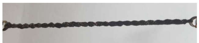
Fig. 2. Image of the polymer actuator coated with the MWCNT/PDMS composite
