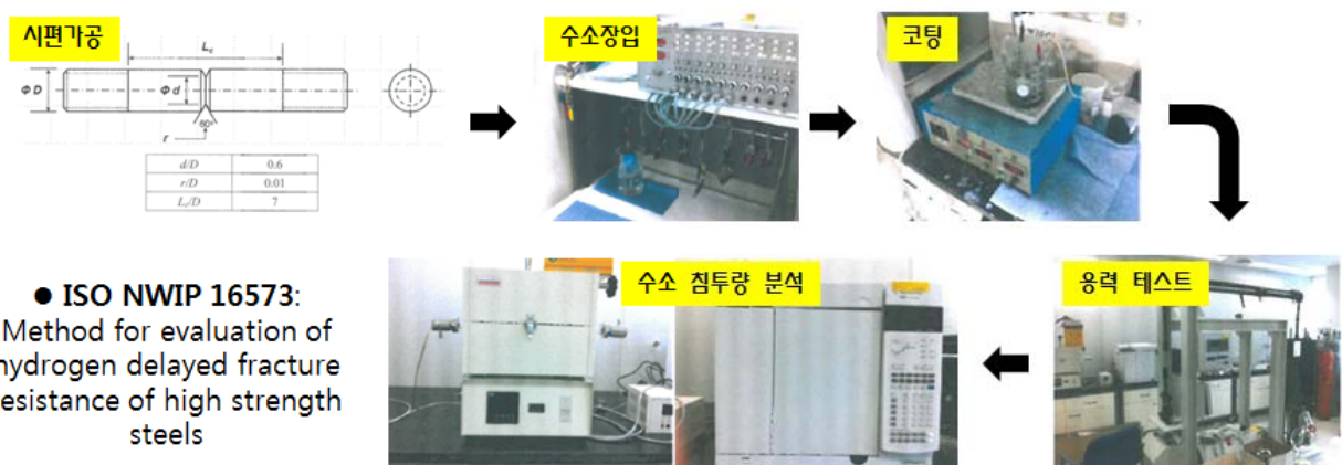
Fig. 3. Process of critical hydrogen contents measurement test
