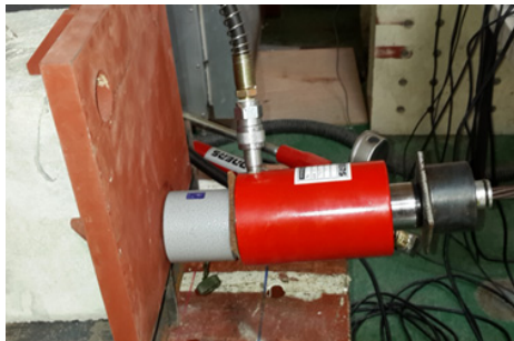
Fig. 9 Details how to introduce tension into tendon specimen
