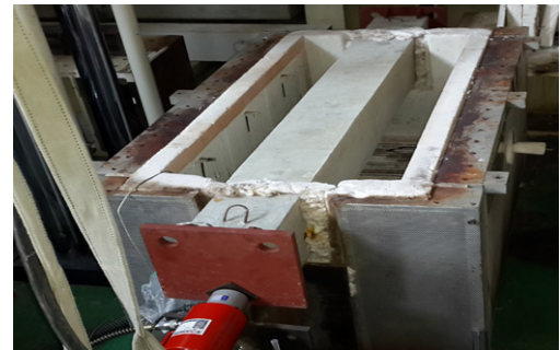
Fig. 6 Set up of post tensioned beam specimen
