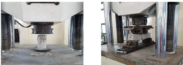
(a) Compressive strength (b) Bending strength
