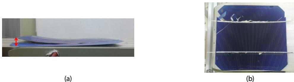
Fig. 1 (a) Bowing and (b) crack issues in thin c-Si solar cells
