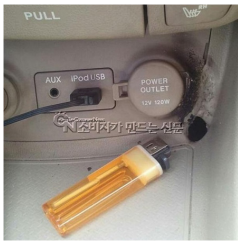
Figure 4. A car fire caused by after-burning of DGL (disposable gas lighter).
