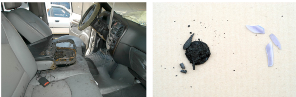
Figure 10. Car fire case due to DGL explosion.
