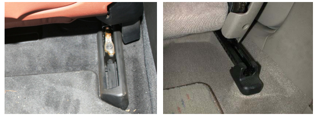
Figure 11. Comparison of blocked and unblocked end of rail protection PVC cover.
