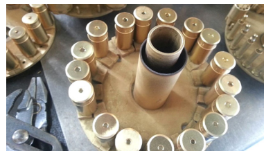
Fig. 5 Spill valve surface treatment process
