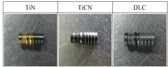
Fig. 8 Used coating spill valve
