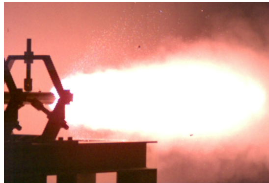
Fig. 7 Ground test of nozzleless booster.
