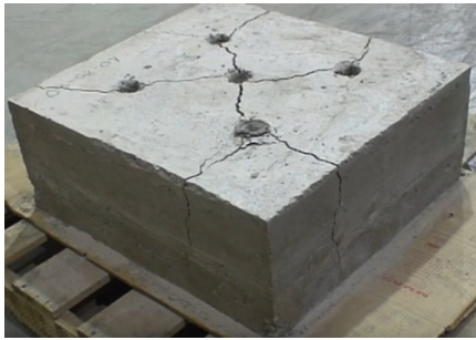
Fig. 1 Concrete demolition using the NEDAs (Archer Company USA, Inc., 2016)
