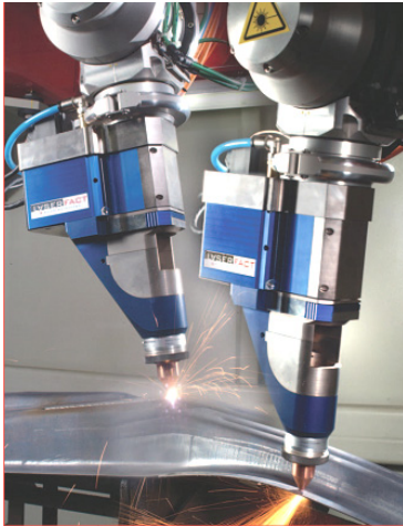
Fig. 3 Combi-head at work. cutting and welding process on the B-pillar with a gantry robot 8)
