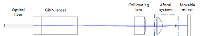
Fig. 7. The whole structure of receiver-transmitter optical system composed of GRIN lens-Collimating lens-Afocal system.
