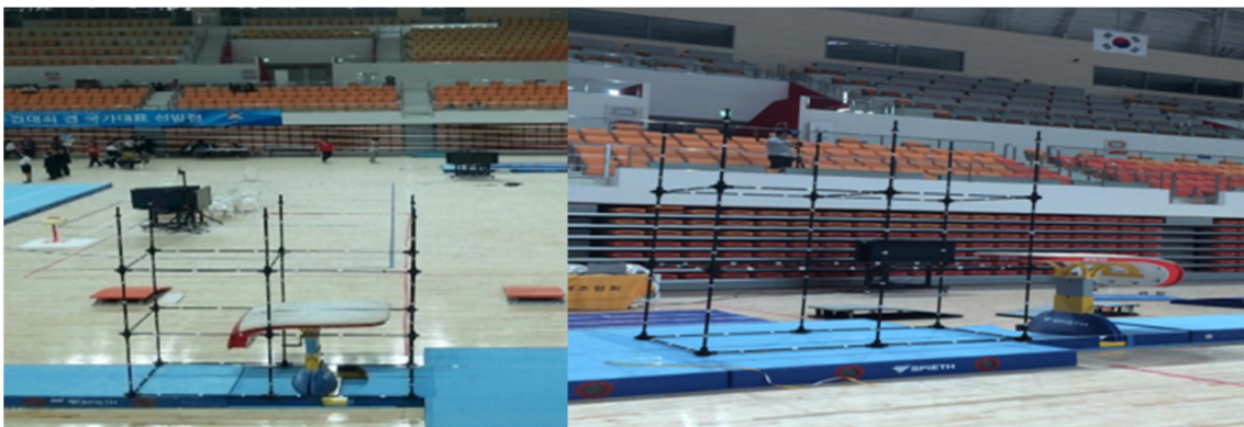
Figure 1. Overview of calibration frame set-up and calibration process before competitions (Park & Kim, 2016)
