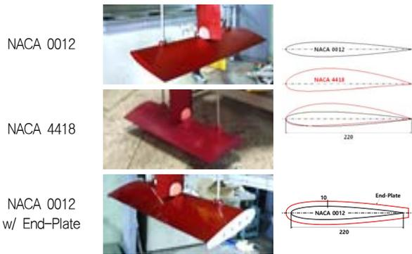
Fig. 9 Different types of hydrofoils
