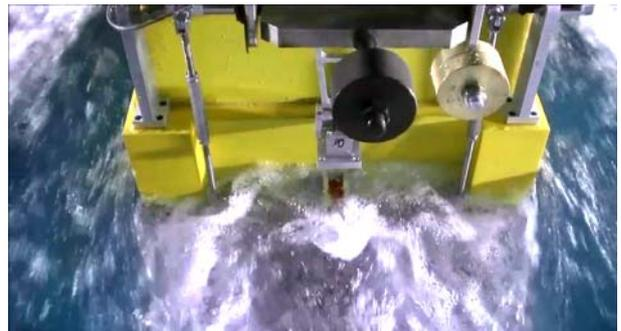
Fig. 7 Photograph taken during resistance test at Vs = 20 km/h
