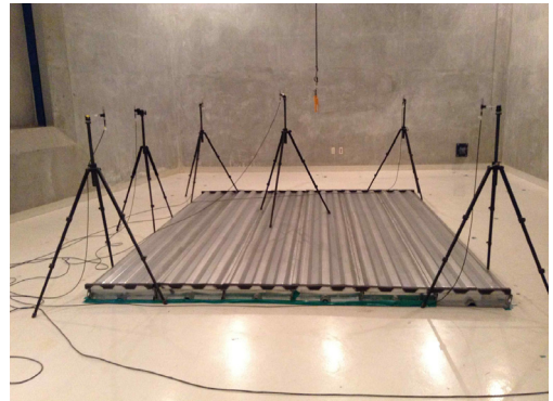
Fig. 1 Example of specimen installation for sound absorption test in reverberation room
