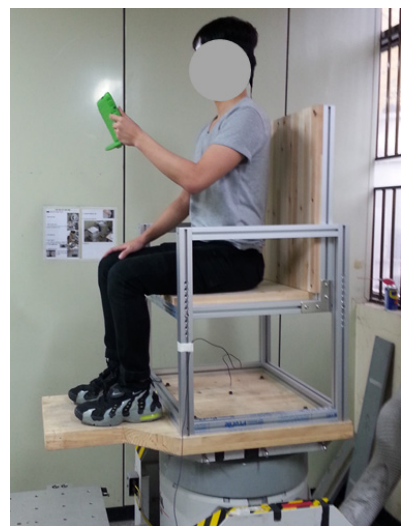
Fig. 3 Rigid seat and sitting posture on the shaker
