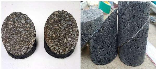
Fig. 2 Specimens for Shear Testing
