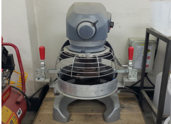
Fig. 10 Wet Track Abrasion Test Machine (A-120)
