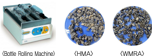
Fig. 2 Samples after Rolling Test
