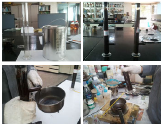
Fig. 4 Storage Stability Test
