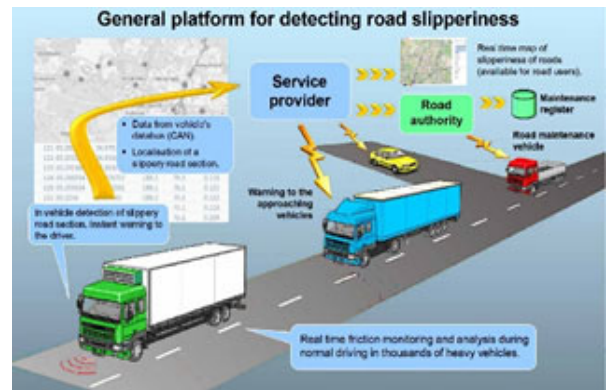
Fig. 1 Slipperiness Detection System in Finland
