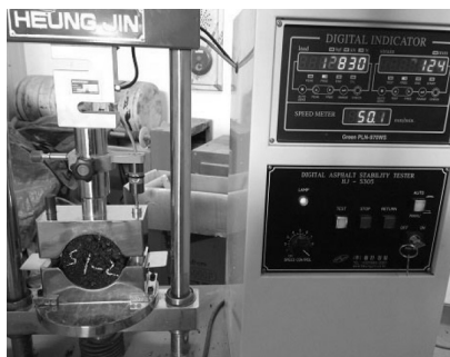
Fig. 4. Measurement of Marshall Stability
