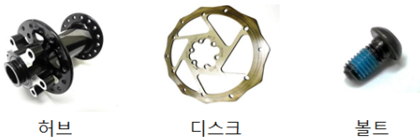
Fig. 3 Fastening system and its components of brake disc
