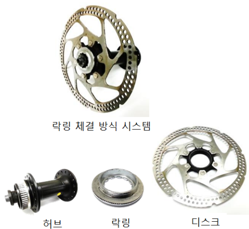
Fig. 6 Brake disc fastening systems and components (lock ring-bolting)
