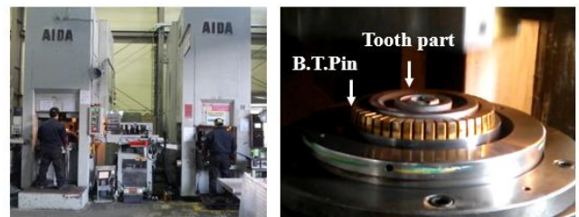
Fig.13 Experiment of cold sizing process for tooth part
