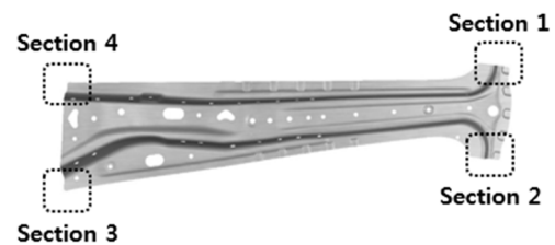
Fig. 9 Section of the center pillar for measuring amount of the springback
