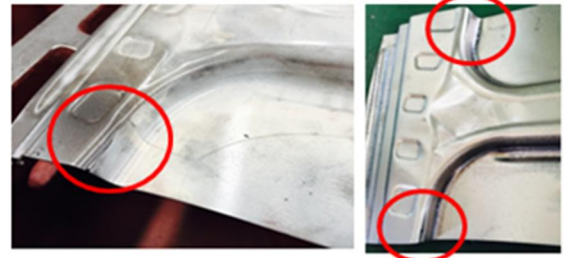
(b) Fracture at edge of the right upper section
