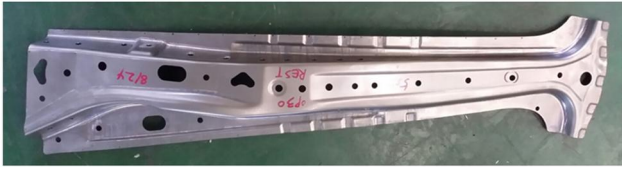
Fig.13 The prototype satisfied with objective of the amount of the spring back (under 0.5mm) at each section
