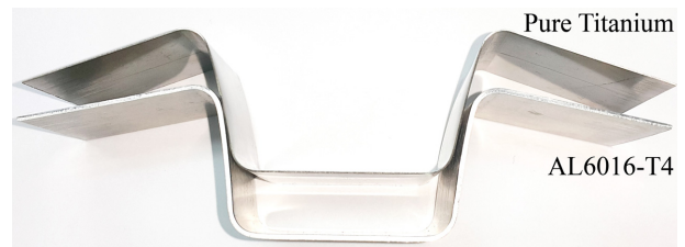
Fig. 6 Experimental results of bending test for CP Ti and Al6016-T4 sheets
