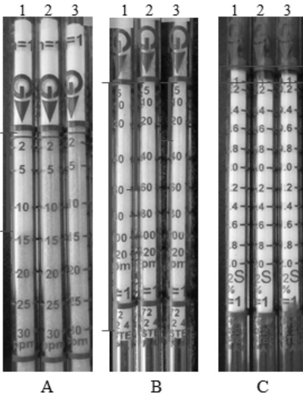
Fig. 4. Total emission of ammonia (A), ethylmercaptan (B), hydrogen sulfide (C) in chicken feces by Lactobacillus sakei treatments. 1, chicken feces; 2, chicken feces + 1/2 Lactobacillus sakei ; 3, chicken feces + Lactobacillus sakei .
