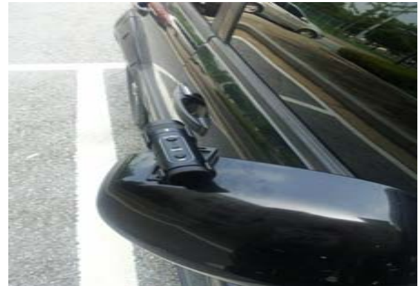
Fig. 3. Side-view mirror camera used in the detection system.
