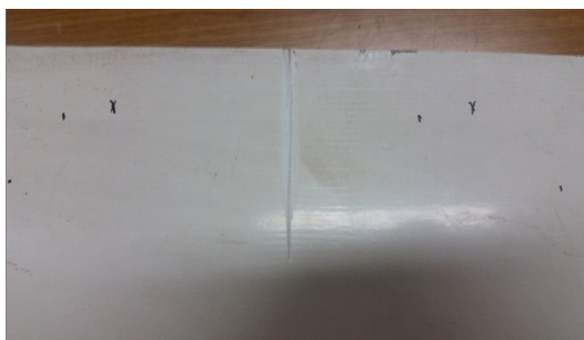
Figure 6. Optical image of blade surface illustrating a crack.
