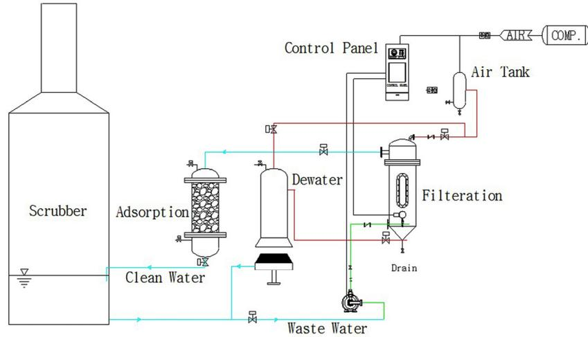
Figure 1. Schematic diagram of scrubber wastewater cleaning system.
