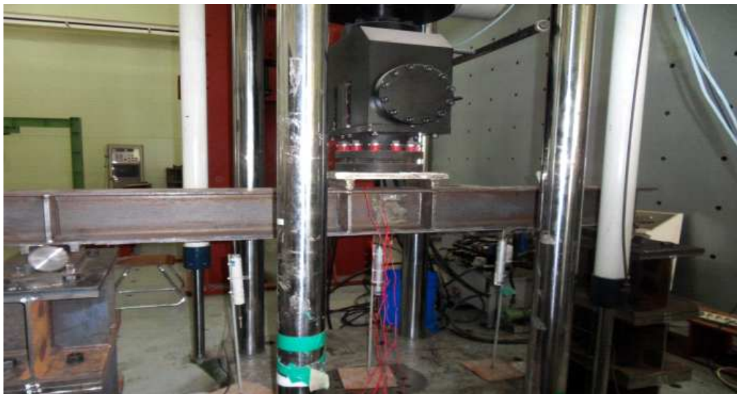
Fig. 1 4-point bending test configuration
