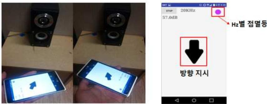
Fig. 4 Smart device detection of signal transmission direction (left), development App configuration (right)
