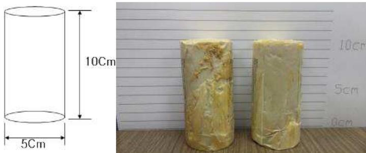
Fig. 2 Compressive Strength Test Specimen
