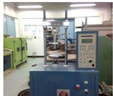
Fig. 3 Apparatus of Compressive Test
