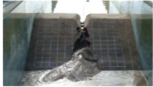
(b) Deep scour progress of vertical wall form
