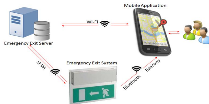
Figure 4. Emergency Exit Management Overall System Architecture
