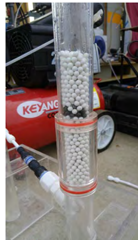
Figure 3: Lab-scale test of reduction catalyst
