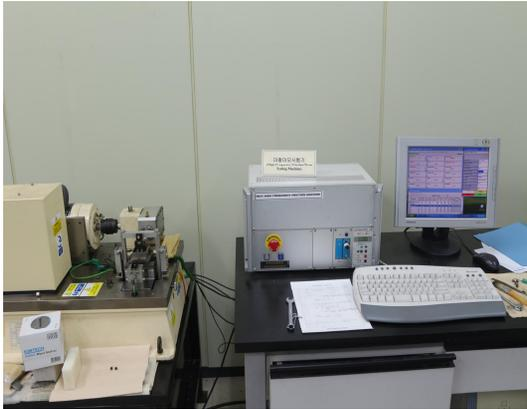
Fig. 2 Equipment of friction tester(TE 77 AUTO)
