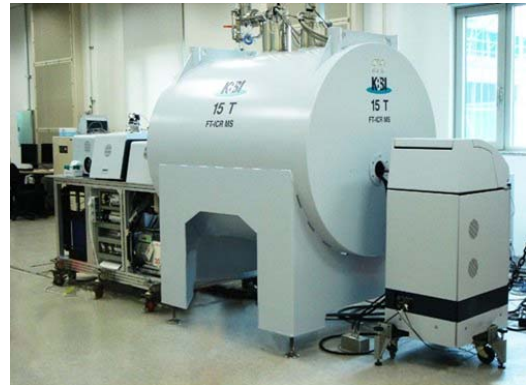
Fig. 2. Fourier transform Ion cyclotron resonance mass spectrometer
