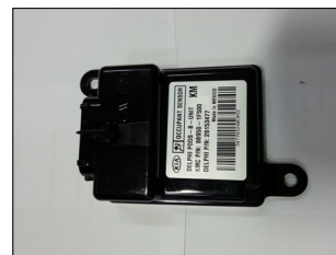
(a) Occupant sensor unit
