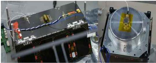
Fig. 7. Mounting accelerometers
